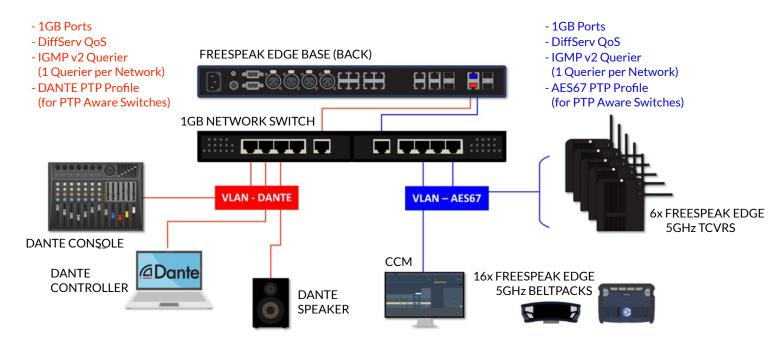
VLAN design and set-up can be very complex. We strongly recommend consulting with a competent IP network engineer in all scenarios where the switch requires specific settings to allow PTP packet forwarding to be of expedited delivery.
